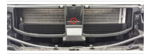
*12.i.* Holding the intercooler radiator up, use the brackets on the left and right sides of the radiator as a guide to drill 6mm holes through the plastic support panel behind (be sure that there are no lines / looms in this position and do not drill through into the AC condenser)
