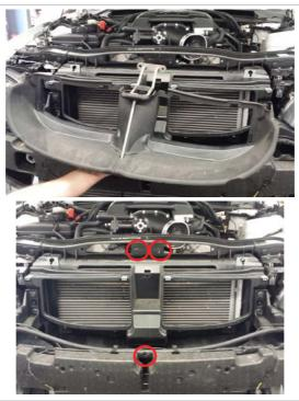
12.f. A 20mm hole is to be drilled in the hood latch recess for mounting the intercooler radiator. Drill the hole 22.5mm from the back face, centered left to right (as shown below). Insert the supplied rubber grommet into the hole.
