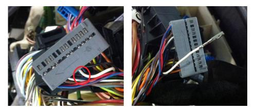
• Solder the Blue DME signal wire to the pin 20 wire where the insulation has been stripped.
