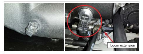
*9.k.* Connect the newly fitted 90 degree quick connect on the idle air circuit hose to the rear L/H side of the supercharger manifold.
