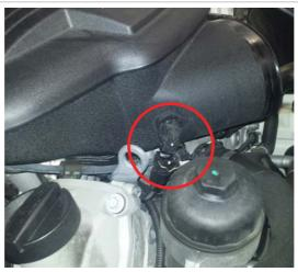
*6.b.* Loosen the 8 hose clamps securing the manifold in place on the throttle bodies.
