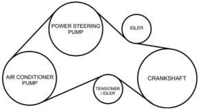
Accessories belt routing for cars produced after 06/2008 with double sided groove belt for air conditioning and power steering pumps.
