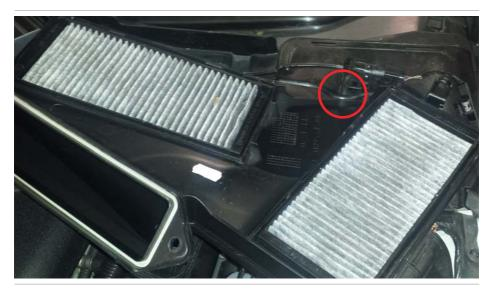
*5.d.* Remove the 3 bolts securing the loom harness. (Found on right hand drive built cars)
