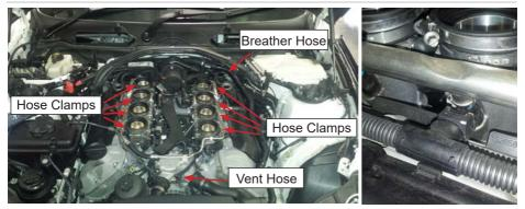
*7.a.* Remove the 4 torx bolts holding the fuel rails, bolts will not be reused.
