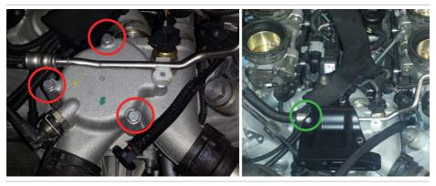
Ensure that the 8 manifold hose clamps are oriented correctly and are loose enough to accept the manifold.
