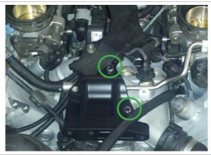
*8.h.* Remove the FEAD assembly (6 by M8 cap screws, be careful not to move the above supercharger FEAD mount) *8.i.* Remove the 4 by M6 cap screws from the fuel rail supercharger mounts.
