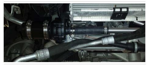
*12.s.* Install the black "Y" fitting into the front intercooler hoses on the supercharger manifold (21mm green band cobra clamps). Install the 420 long 19mm hose to the other end of the "Y" piece fitting and secure with a cobra clamp (white band).
