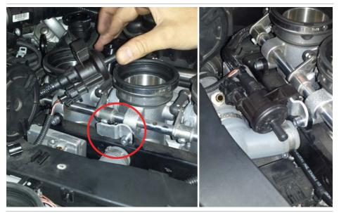
*7.i.* Use the supplied zip tie to secure the purge solenoid to the mounting bracket.
