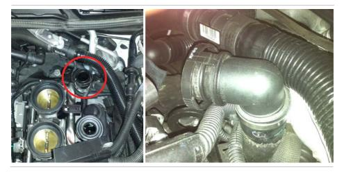
*7.I.* Remove the engine lifting bracket from the front R/H side of the engine, shown in green, this will not be refitted (2 x 8mm torx bolts). The breather line located at the front L/H side of the engine requires shortening (shown in red below). Trim 75mm off the end of this hose.
