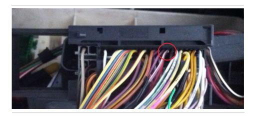
• Slide the locking mechanism for the main connector out.
