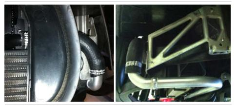
12.p. Install the 125 long 19mm hose to the straight end of the long intercooler pipe using a cobra clamp (white band).
