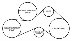
*11.b.* Remove the main drive belt (this requires removal of the idler pulley next to the water pump pulley).
