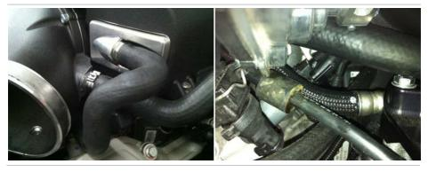
*9.e.* Visually check that the rubber throttle body boots are in the correct position and are not folded.
