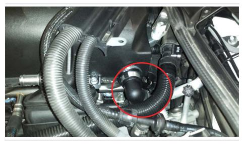
*9.1.* Install the supplied valve cover molded breather hoses to the valve covers / supercharger inlet as shown below. Secure with 4 cobra clamps (black band).
