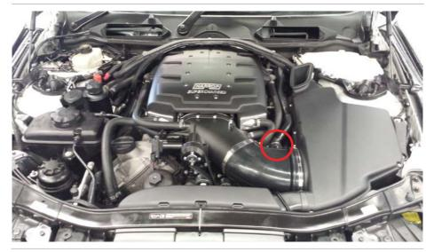
**21.** Re-install all ancillary components that were removed during the supercharger installation (strut braces, accessories cover, fresh air filters etc).
