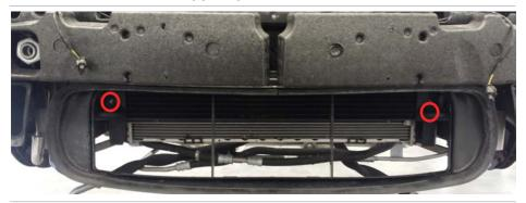
*12.k.* Install intercooler pipe to the R/H side of the intercooler radiator using the supplied M6 button head / flange nut.
