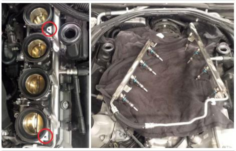
7.b. Remove the injector clips and injectors from fuel rails. Caution: Use eye protection when removing injectors. The system is still pressurized and may squirt fuel as the first injector is removed. Use a suitable method to collect fuel. Lubricate o-rings on new injectors and install into fuel rails. Secure injectors with factory clips.
