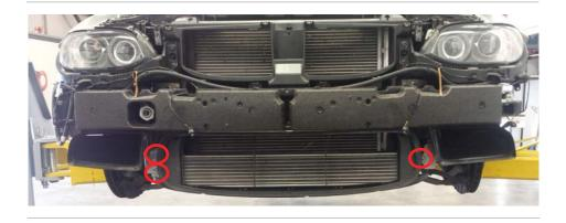
*12.h.* Install the intercooler radiator by sliding it up from under the vehicle until the pin is fully inserted in the grommet installed previously. The bleeder nipple should be on the R/H side of the car.
