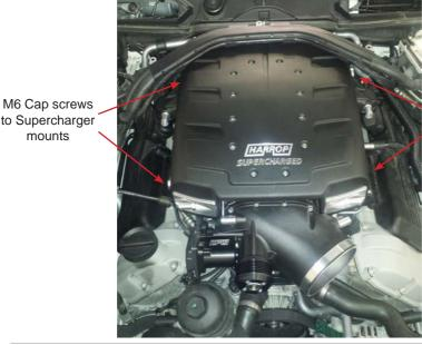
M6 Cap screws to Supercharger mounts
