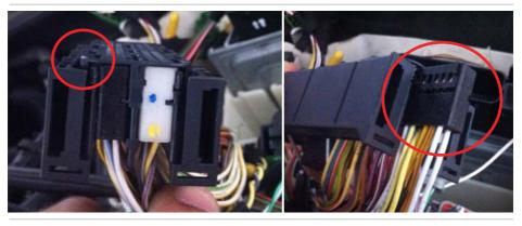
• Remove the wire located in pin 37 from the sub connector. Strip 10mm of insulation off the wire 50mm back from the pin.
