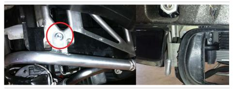
*12.I.* Loosen the 2 nuts above and the 2 nuts below on the R/H side of the radiator that mount the radiator support panel to the sub fame.
